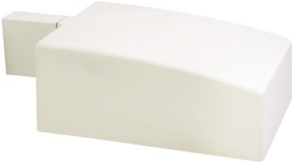
Type II distribution Area Light with pole top fixed arm mount for use on 10' - 15' poles. Fixed mounting at 90° to pole. Drilling 2" on center. Factory wired for 277V. Lamp supplied.
