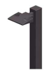
ALED Area Light mounts to 4" square steel poles at 15-20'. 1 to 4 ALEDs can be mounted to each pole. IESNA Full Cutoff, Fully shielded optics. 5 year warranty.
