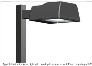
Type II distribution Area Light with pole top fixed arm mount. Fixed mounting at 90° to pole. Drilling 2" on center. Factory wired for 277V. Lamp supplied.
