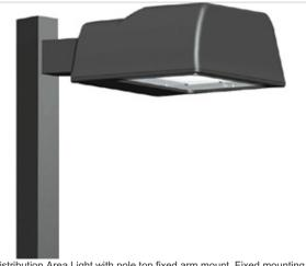
Type II distribution Area Light with pole top fixed arm mount. Fixed mounting at  $90^{\circ}$  to pole. Drilling 2" on center. Factory wired for 277V. Lamp supplied.
