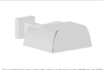
Type II distribution Area Light with wall mount. Fixed mounting @  $90^{\circ}$  to wall. Drilling 2" on center. Factory wired for 277V. Lamp supplied.
