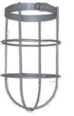
Flat or round bottom wire clamp guard made of No. 8 gauge steel rod welded to a clamping band. Guard is protected from corrosion by a baked silver gray polyester powder finish.
