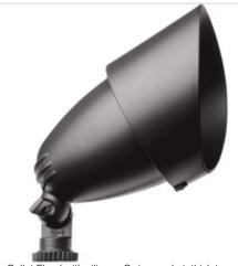
75 Watt Quartz Bullet Flood with silicone O-ring gasket, thick tempered glass lens, internal and external cooling fins. Gold plated socket contacts and 250°C Teflon coated wires for extended lamp life. Lamp supplied.
