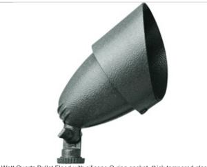
75 Watt Quartz Bullet Flood with silicone O-ring gasket, thick tempered glass lens, internal and external cooling fins. Gold plated socket contacts and 250°C Teflon coated wires for extended lamp life. Lamp supplied.
