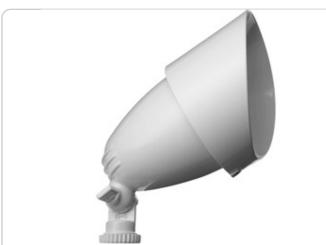
75 Watt Quartz Bullet Flood with silicone O-ring gasket, thick tempered glass lens, internal and external cooling fins. Gold plated socket contacts and 250°C Teflon coated wires for extended lamp life. Lamp supplied.
