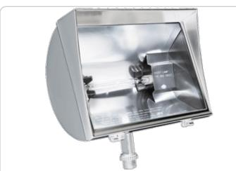
Sleek design 500 Watt Quartz flood with rounded back and fins for superior heat dissipation. Vandalproof stainless steel locking clip. Gold plated socket contacts and 250°C Teflon coated wires for extended lamp life. Lamp supplied.
