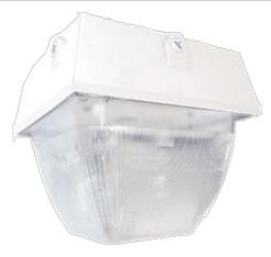
Large size ceiling mount fixture. Vertical lamp HID. Adjustable, 4-way glare guard & "No Bend" conduit entrance. Excellent heat control eliminates heat problems. Housing is die cast aluminum with clear vandalproof polycarbonate refractor. Lamps supplied.
