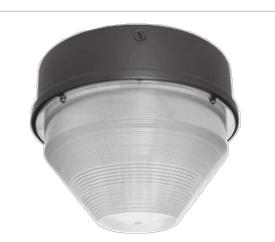
15" round die cast aluminum housing with vandalproof refractor for optimum parking garage light distribution. 150 or 175 w vertical mount Metal Halide or 100,000 hour Induction. Lamp supplied.
