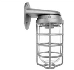
Die cast aluminum construction with sturdy wall mounting bracket. Medium base socket and a variety of globes. incandescent lamp A21 for 100 Series, PS25 for 200 Series. Lamp not supplied.
