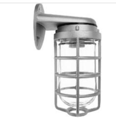
Die cast aluminum construction with sturdy wall mounting bracket. Medium base socket and a variety of globes. incandescent lamp A21 for 100 Series, PS25 for 200 Series. Lamp not supplied.
