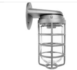
Die cast aluminum construction with sturdy wall mounting bracket. Medium base socket and a variety of globes. incandescent lamp A21 for 100 Series, PS25 for 200 Series. Lamp not supplied.
