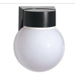
Entry light in 50 Watt HP. Cast aluminum housing with decorative white glass globe or unbreakable polycarbonate. Bracket fixture mounts to common junction boxes. Photocell models available. Minimum operating temperature 14°F, HPS lamps supplied.
