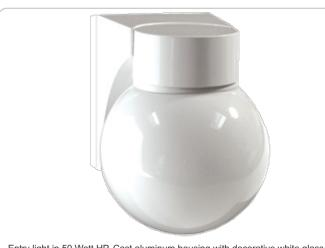
Entry light in 50 Watt HP. Cast aluminum housing with decorative white glass globe or unbreakable polycarbonate. Bracket fixture mounts to common junction boxes. Photocell models available. Minimum operating temperature 14°F, HPS lamps supplied.
