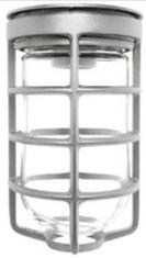
Die cast aluminum construction. Mounts to existing surface or recessed 4" boxes. Adapter plate provided. Medium base socket and a variety of globes. Lamp supplied.
