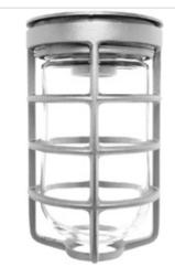
Die cast aluminum construction. Mounts to existing surface or recessed 4" boxes. Adapter plate provided. Medium base socket and a variety of globes. incandescent lamp A21 for 100 Series, PS25 for 200 series. Lamp not supplied.
