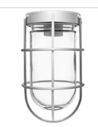
Die cast aluminum construction. Mounts to existing surface or recessed 4" boxes. Adapter plate provided. Medium base socket and a variety of globes. incandescent lamp A21 for 100 Series, PS25 for 200 series. Lamp not supplied.
