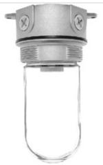
Box mount, die cast aluminum with built-in junction box and sturdy mounting lugs. Medium base socket, 1/2" or 3/4" NPS hub size and a variety of globes. incandescent lamp A21 for 100 Series, PS25 for 200 Series. Lamp not supplied.
