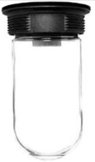
Box mount, die cast aluminum with built-in junction box and sturdy mounting lugs. Medium base socket, 1/2" or 3/4" NPS hub size and a variety of globes. incandescent lamp A21 for 100 Series, PS25 for 200 Series. Lamp not supplied.
