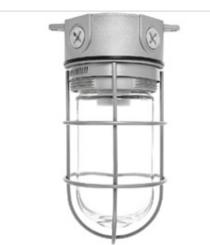
Box mount, die cast aluminum with built-in junction box and sturdy mounting lugs. Medium base socket, 1/2" or 3/4" NPS hub size and a variety of globes. incandescent lamp A21 for 100 Series, PS25 for 200 Series. Lamp not supplied.
