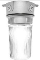
Box mount, die cast aluminum with built-in junction box and sturdy mounting lugs. Medium base socket, 1/2" or 3/4" NPS hub size and a variety of globes. incandescent lamp A21 for 100 Series, PS25 for 200 Series. Lamp not supplied.
