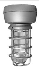
Cast aluminum housing for 50, 70 & 100 Watt HPS and MH. Prismatic globe for low glare and even light distribution. Fixture mounts to junction box or can be wired inside the housing. Ceiling mounted with 1/2" NPS(or 3/4") side and top conduit feed. Lamp supplied.
