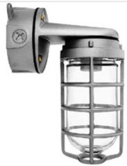
Die cast aluminum construction. Wall bracket plus junction box with sturdy mounting lugs. Medium base socket, 1/2" or 3/4" NPS hub size and a variety of globes. Lamp supplied.
