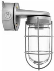
Die cast aluminum construction. Wall bracket plus junction box with sturdy mounting lugs. Medium base socket, 1/2" or 3/4" NPS hub size and a variety of globes. incandescent lamp A21 for 100 series, PS25 for 200 Series. Lamp not supplied.
