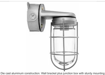
Die cast aluminum construction. Wall bracket plus junction box with sturdy mounting lugs. Medium base socket, 1/2" or 3/4" NPS hub size and a variety of globes. Lamp supplied.
