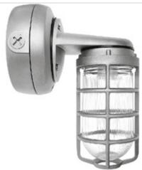
Small cast aluminum housing with study wall mounting bracket for 13 and 26 Watt or larger size housing for 32 and 42 compact fluorescent. Prismatic globe for low glare and even light distribution. Fixture mounts to junction box or can be wired inside the housing. Wall mounted with 1/2" NPS(or 3/4") side and top conduit feed. Lamp supplied.
