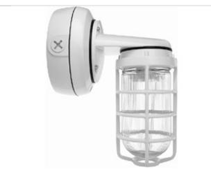
Small cast aluminum housing with study wall mounting bracket for 13 and 26 Watt or larger size housing for 32 and 42 compact fluorescent. Prismatic globe for low glare and even light distribution. Fixture mounts to junction box or can be wired inside the housing. Wall mounted with 1/2" NPS(or 3/4") side and top conduit feed. Lamp supplied.
