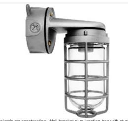
Die cast aluminum construction. Wall bracket plus junction box with sturdy mounting lugs. Medium base socket, 1/2" or 3/4" NPS hub size and a variety of globes. incandescent lamp A21 for 100 series, PS25 for 200 Series. Lamp not supplied.
