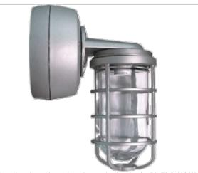
Cast aluminum housing with sturdy wall mounting bracket for 50, 70 & 100 Watt HPS, 50, 70, 100 Watt Metal Halide. Prismatic globe for low glare and even light distribution. Fixture mounts to junction box or can be wired inside the housing. Wall mounted with 1/2" NPS (or 3/4") side and top conduit feed. Lamp supplied. Weight: 10.3 lbs
