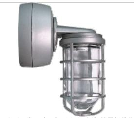
Cast aluminum housing with sturdy wall mounting bracket for 50, 70 & 100 Watt HPS, 50, 70, 100 Watt Metal Halide. Prismatic globe for low glare and even light distribution. Fixture mounts to junction box or can be wired inside the housing. Wall mounted with 1/2" NPS (or 3/4") side and top conduit feed. Lamp supplied.
