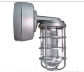
Cast aluminum housing with sturdy wall mounting bracket for 50, 70 & 100 Watt HPS, 50, 70, 100 Watt Metal Halide. Prismatic globe for low glare and even light distribution. Fixture mounts to junction box or can be wired inside the housing. Wall mounted with 1/2" NPS (or 3/4") side and top conduit feed. Lamp supplied.
