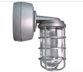
Cast aluminum housing with sturdy wall mounting bracket for 50, 70 & 100 Watt HPS, 50, 70, 100 Watt Metal Halide. Prismatic globe for low glare and even light distribution. Fixture mounts to junction box or can be wired inside the housing. Wall mounted with 1/2" NPS (or 3/4") side and top conduit feed. Lamp supplied. Weight: 11.8 lbs
