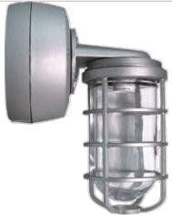
Cast aluminum housing with sturdy wall mounting bracket for 50, 70 & 100 Watt HPS, 50, 70, 100 Watt Metal Halide. Prismatic globe for low glare and even light distribution. Fixture mounts to junction box or can be wired inside the housing. Wall mounted with 1/2" NPS (or 3/4") side and top conduit feed. Lamp supplied.
