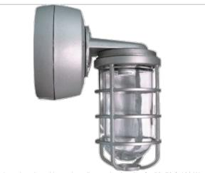
Cast aluminum housing with sturdy wall mounting bracket for 50, 70 & 100 Watt HPS, 50, 70, 100 Watt Metal Halide. Prismatic globe for low glare and even light distribution. Fixture mounts to junction box or can be wired inside the housing. Wall mounted with 1/2" NPS (or 3/4") side and top conduit feed. Lamp supplied. Weight: 7.7 lbs
