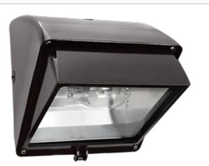
Cutoff Wallpack with glare shield for 35 - 100W HPS, 50 - 100W MH (Pulse Start Standard) or 42W CFL. Lens is flat, tempered glass.  $30^{\circ}$ . cutoff strip included. Lamp supplied.
