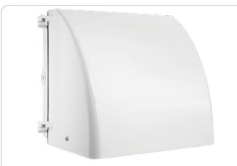
Fully shielded, Full Cutoff compact Wallpack for higher Wattages! 150W HPS & 125W QT P.S. MH. Full Cutoff optics with flat tempered glass lens. Cap/Ignitor cradle and EZ mount knockouts for easy wiring. Lamp supplied.
