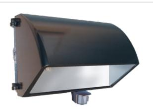
Sensor controlled WP2 Wallpack in 42 Watt CFL cutoff & 84 Watt CFL refractor models. Starting temperature 0°F/-18°C. Sensor has 180°detection and controls up to 250 Watts. 120 volts only. Lamp supplied.
