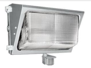
Sensor controlled mid size Wallpack for up 84 Watts compact fluorescent @ 120v. Sensor has  $180^{\circ}$  detection Sensor color matched to fixture. Minimum starting temperature  $0^{\circ}$ F. Lamps supplied.
