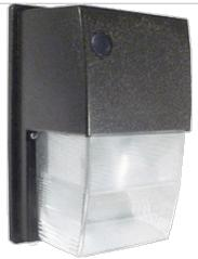
28 thru 42 Watt compact fluorescent Tallpack. Vandal resistant polycarbonate housing. Heavy die-cast aluminum back plate with 1/2" bottom and back conduit opening. Factory installed 120V photocell with bypass cap included. Operating temperature 28w (-20°F), 26, 32 & 42w(0°F). Lamp supplied.
