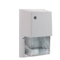
Heavy duty die cast aluminum housing with prismatic glass refractor. HPS and Metal Halide models available with 1/2" bottom and back conduit opening. Factory installed photocell optional. Lamp supplied.
