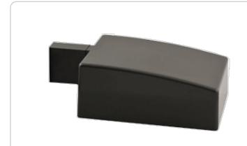
Type II distribution Area Light with pole top fixed arm mount for use on 10' - 15' poles. Fixed mounting at  $90^\circ$  to pole. Drilling 2'' on center. Factory wired for 277V. Lamp supplied.
