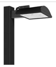
Specification grade area lights available in IES Type II distributions. For use in parking lots, roadways, pathways and general area lighting. Mounts to 4" square steel poles at 20-35'. Includes built in support for Lightcloud, a wireless lighting control system and service, fully developed by RAB. 5 Year Warranty
