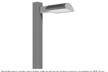
Specification grade area lights with multi-level motion sensor available in IES Type III distributions. For use for roadway, general parking and other area lighting applications where a larger pool of lighting is required. Mounts to 4" square steel poles at 20-35'. Patent pending thermal management system. 5 Year Warranty.
