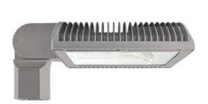
Specification grade area lights available in IES Type III distributions. For use for roadway, general parking and other area lighting applications where a larger pool of lighting is required. Mounts to 4" square steel poles at 20-35'. Patent pending thermal management system. 5 Year Warranty.
