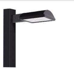
Specification grade area lights available in IES Type IV distributions. Suited for mounting on the sides of buildings and walls, and for illuminating the perimeter of parking areas. Mounts to 4" square steel poles at 20-35'. Patent pending management system. 5 Year Warranty.
