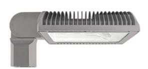
Specification grade area lights available in IES Type IV distributions. Suited for mounting on the sides of buildings and walls, and for illuminating the perimeter of parking areas. Mounts to 4" square steel poles at 20-35'. Patent pending management system. 5 Year Warranty.
