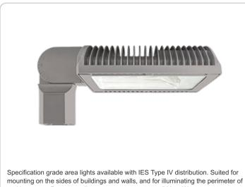
Project: Type: Prepared By: Date: **Driver Info** LED Info Type: Constant Current Watts: 78W 120V: 0.66A Color Temp: 3000K 208V: 0.41A Color Accuracy: 82 CRI 240V: 0.35A L70 Lifespan: 100000 277V: 0.30A 5,968 Lumens: Input Watts: 79W Efficacy: 75 LPW Efficiency: 98%
